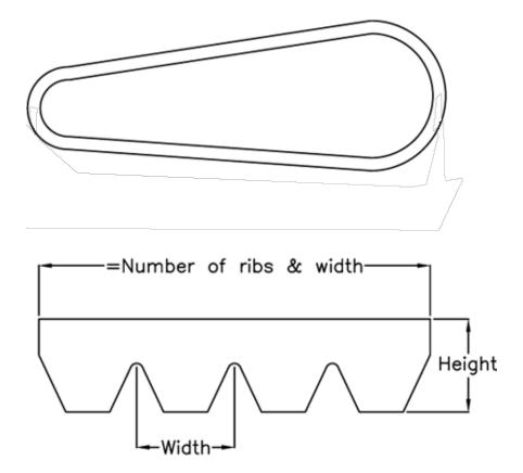
$\begin{array}{ll} \text{Datum Llength} = 2705 \\ \text{Height} &= 9.5 \\ \text{Number of ribs} = 6 \\ \text{Pitch} &= 4.7 \end{array}$
